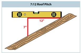
Roof pitch (slope really, but it is known as pitch) refers to the amount of **rise** a roof has compared to the horizontal measurement of the roof. The picture opposite shows the pitch of a 7:12 roof slope meaning that for 12" of horizontal measurement (roof run) the vertical measurement (roof rise) is 7". This measurement is best done on a bare roof, but If this isn't practical then perform the same measurement on the underside of the roof (loft).
